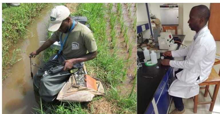
Figure 10. Measuring water parameters at the field using HQ40d multimeter, IntelliCAL PHC101 probe, and HACH LDO probe (Left), and laboratory analysis of Phosphate, Nitrate, and Turbidity (right).
