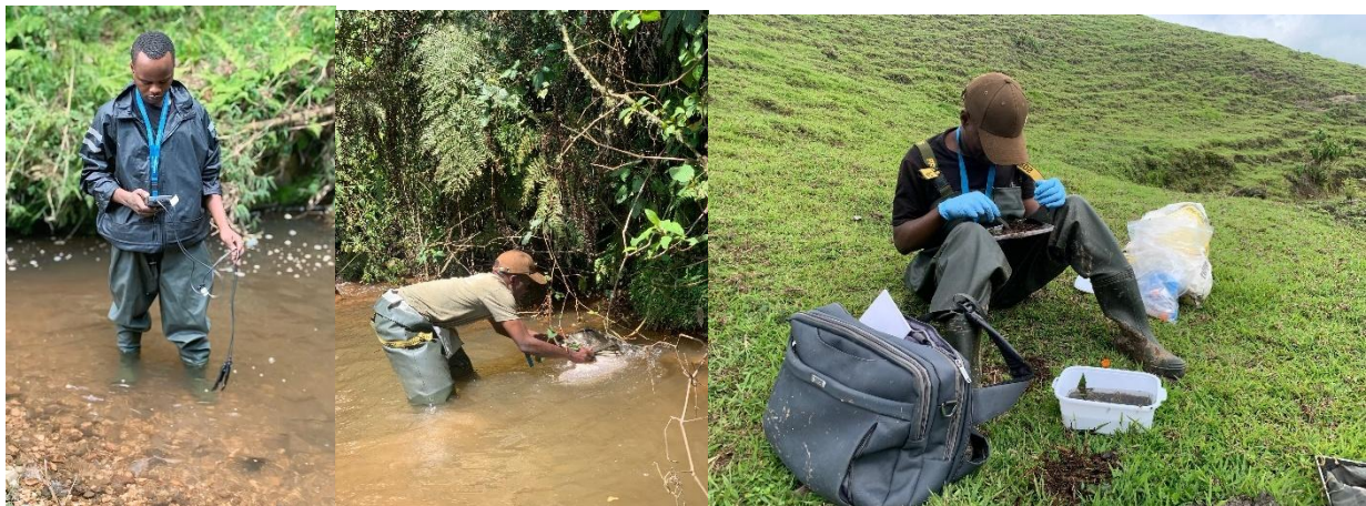
Figure 3: Measurement of water quality and sampling of water macroinvertebrates
